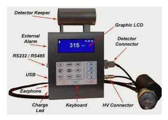
The internal RAM can store up to 20 energy spectra, which can be downloaded to a PC by a RS232/RS485 or USB connection.
